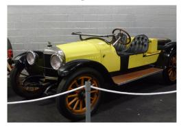
Some basic facts: Chassis Number: L72676 Horsepower: 39 Displacement: 4-cylinder, 3.15 liter Wheel Base: 112"
