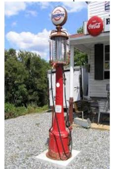
From there, it was easy to imagine the pump and glass cylinder integrated into one unit. In 1917, the Wayne Pump Company offered the first self-contained "visible measure" pump designed as a single unit. Within two years, other manufacturers offered such units and most major oil companies were specifying same. These so-called "visible" gas pumps came into standard use throughout the 1920s. A visible gas pump is shown at the right.
