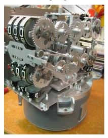
Root Company. Thus, Veeder Root Company manufactured and sold the Veeder Root computer to <u>all</u> manufacturers of gas pumps from the late 1940s into the early 1960s. While I have three different brands of gas pumps (see below) in my collection, all of my pumps have Veeder Root calculators. Of course, the age of transistors brought fully electric calculators and made the Veeder Root calculator obsolete. Still, it was a good run.
