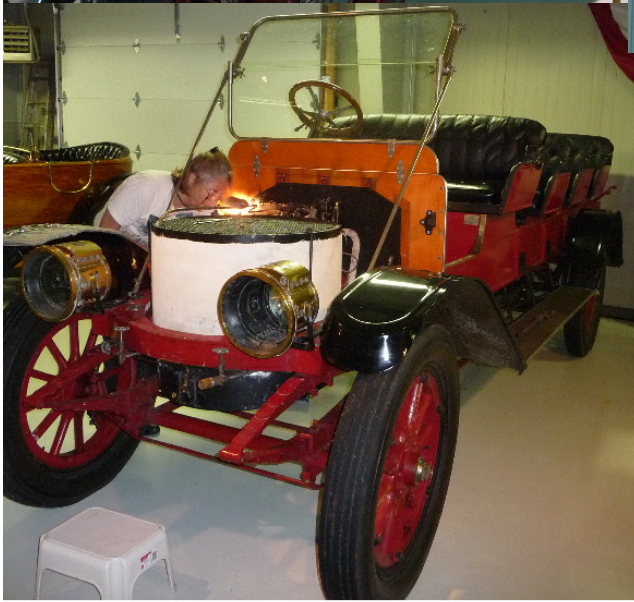
1914 Stanley Steamer 14 passenger Mountain Wagon; note the new boiler and lady redoing the piping
